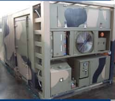
20ft refrigerated container with removable genset
